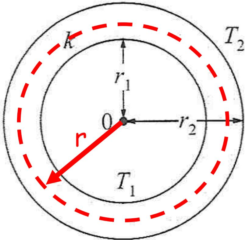
$$- \int_{r_1}^{r_2} \frac{dr}{r^2} = \frac{k 4 \pi}{\alpha} \int_{T_1}^{T_2} dT$$
