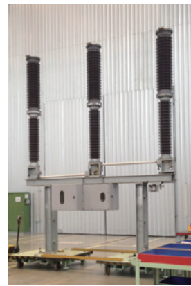
145kV 3-Phase GCB
