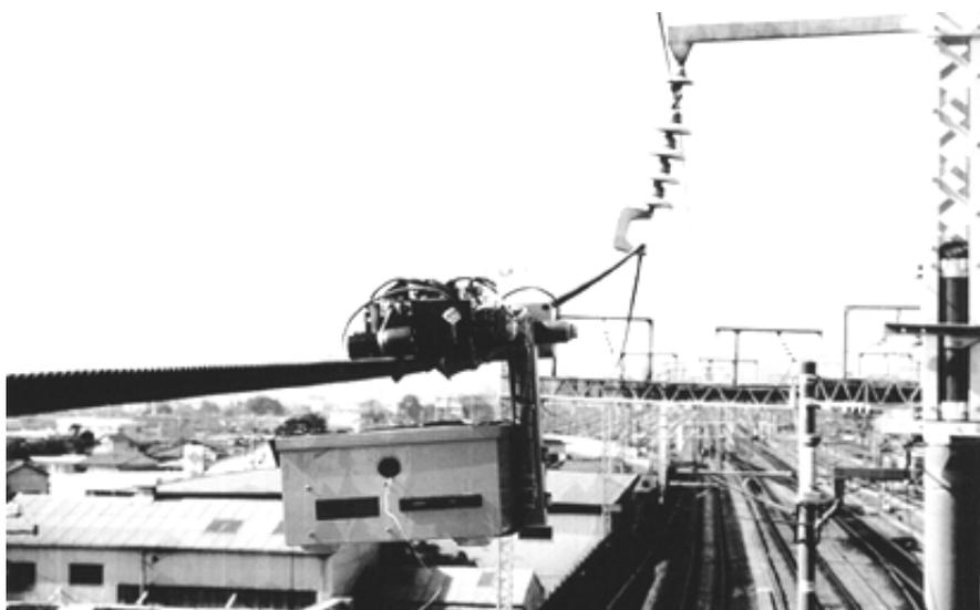
Feeder line inspection robot
