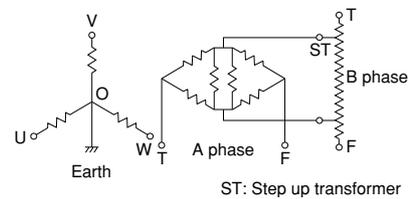
**Figure 7 Structure of an AC Feeding System**
