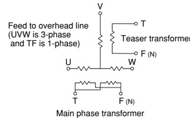
**Figure 6 Modified Wood-bridge Connected Transformer**
