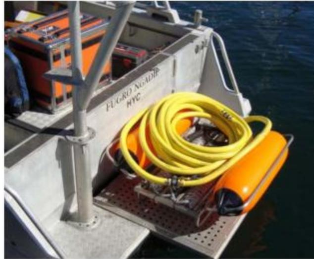
*Fig. 1 Multi-tip sparker, cable and floaters (© Geo Resources)*
