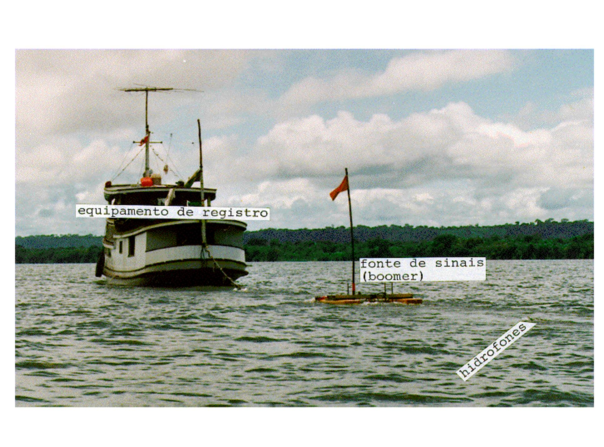
A photograph of a boat on a lake. The boat is on the left side of the frame, with a mast and rigging. In the middle ground, there is a small buoy with a red flag on a pole, labeled as a boomer. In the bottom right corner, there is a label for hydrophones. The background shows a forested shoreline under a cloudy sky.
