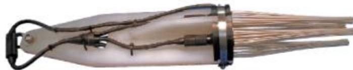
*Fig. 2 "Squid-like" sparker source (© Applied Acoustics)*
