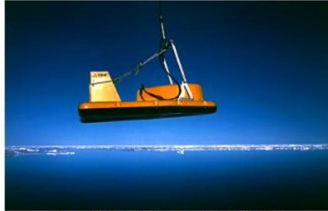
*Fig. 1 Typical Chirp towfish (© EG&G)*
