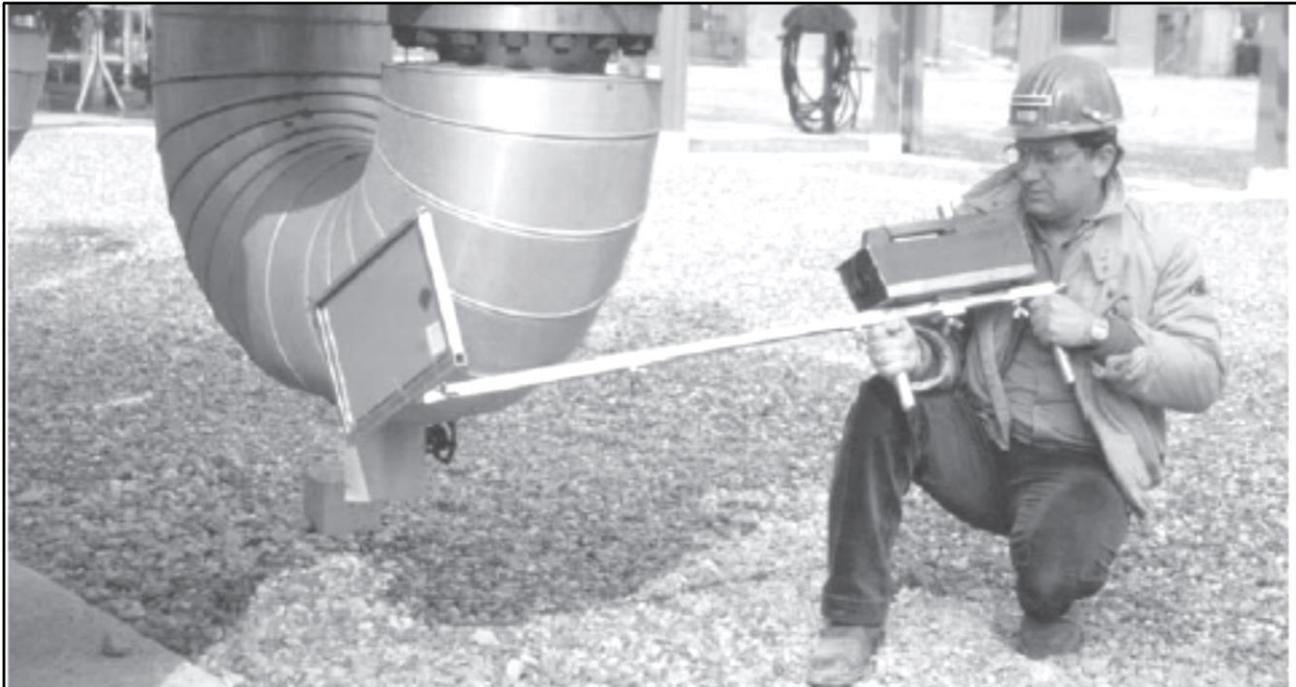
*Fig. 10-18. Flash radiography of an insulated pipe section*
