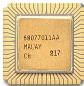
**Figura 5.9 Encapsulamento LCCC.**
