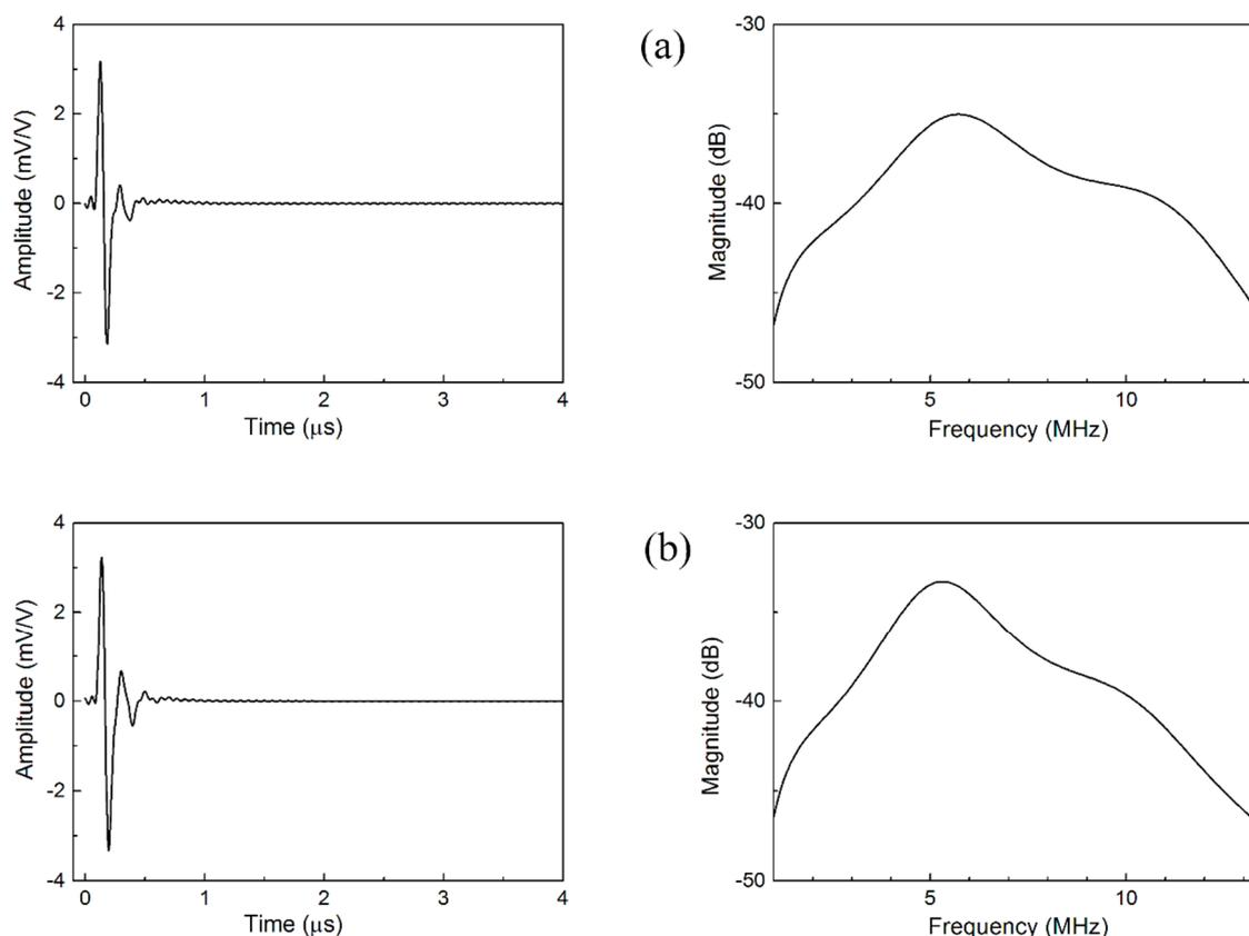
**Figure 3.** The simulated waveforms and frequency spectra of the designed TOFD ultrasonic transducers with (a) scheme I; (b) scheme II.
