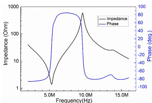
**Figure 2.** The impedance and phase angle spectra of the prepared PMNT/epoxy 1–3 composite.
