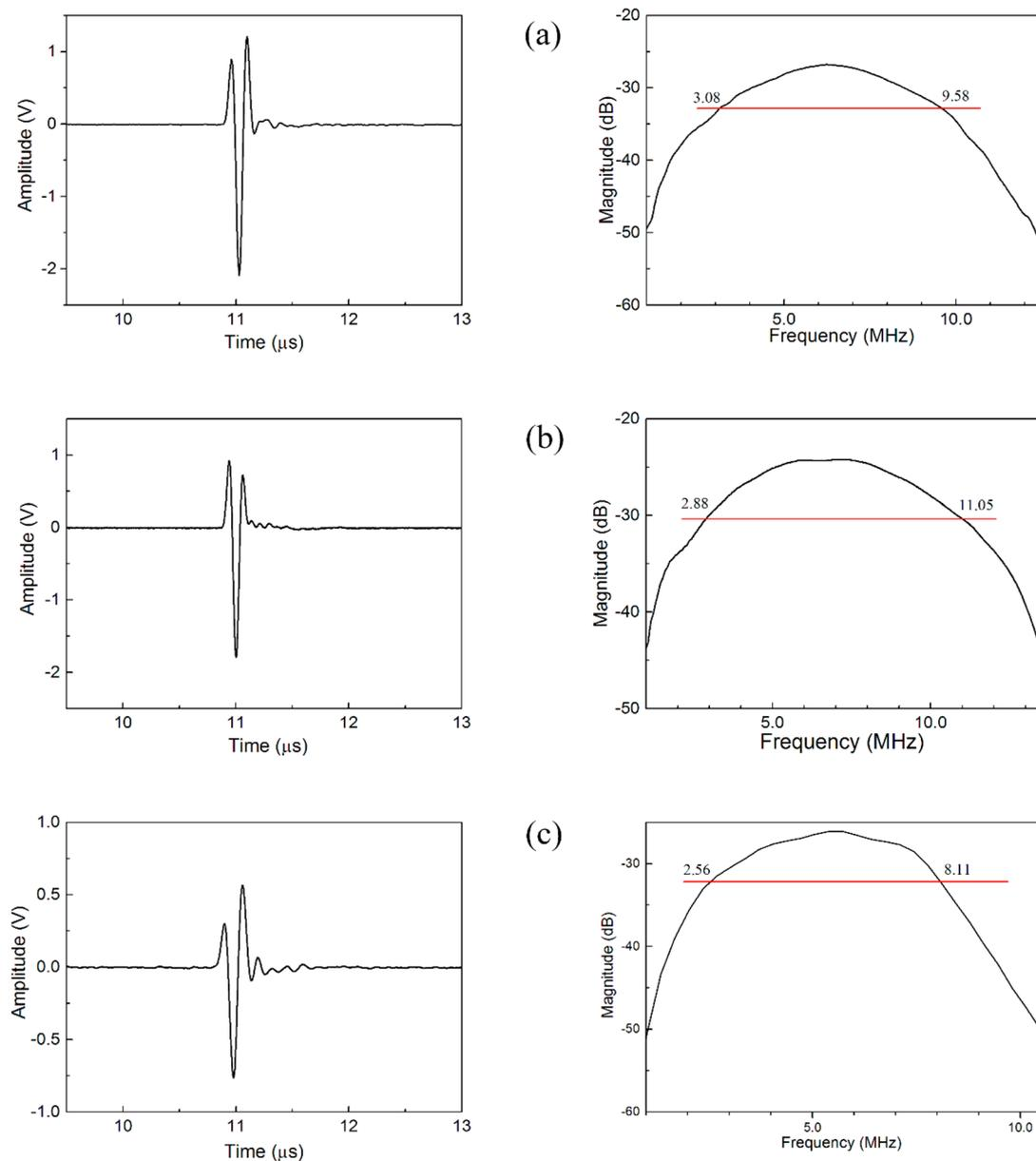
**Figure 5.** Comparison of the waveforms and frequency spectra of (a) PMNT/epoxy 1–3 composite TOFD ultrasonic transducers with scheme I; (b) PMNT/epoxy 1–3 composite TOFD ultrasonic transducers with scheme II, and (c) PZT/epoxy 1–3 composite TOFD ultrasonic transducers.
