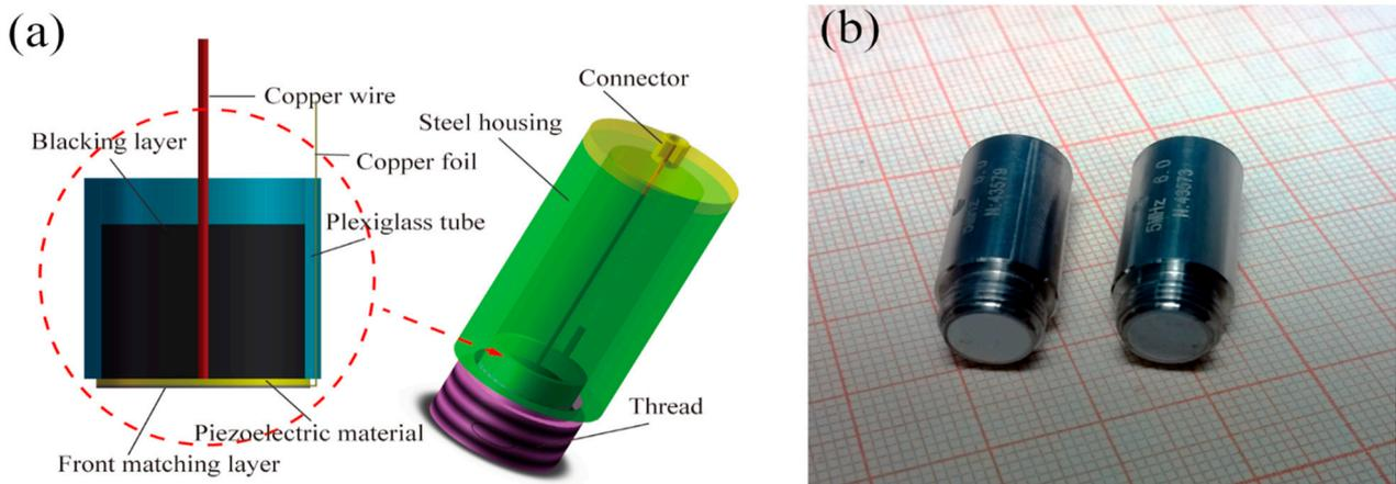
**Figure 4.** (a) Schematic diagram of the designed TOFD ultrasonic transducer; (b) Photograph of the fabricated TOFD ultrasonic transducer.
