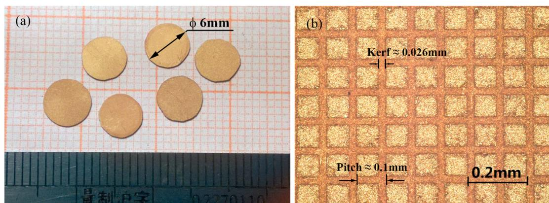
**Figure 1.** (a) Photograph of the prepared PMNT/epoxy 1–3 composites; (b) Enlarged image of a randomly selected area on the composite.
