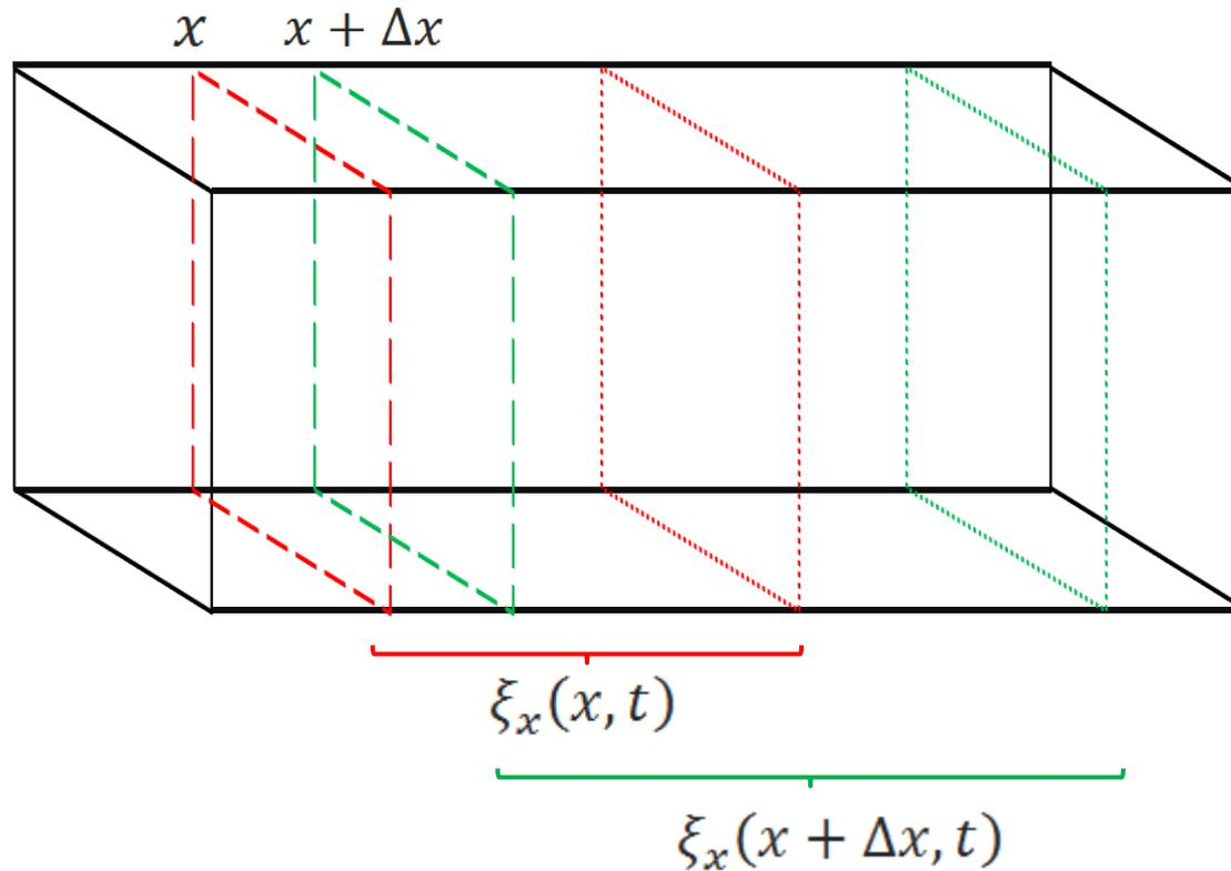
$$V = A[(x + \Delta x) - x] \quad V + \Delta V = A\{\Delta x + [\xi_x(x + \Delta x, t) - \xi_x(x, t)]\}$$
