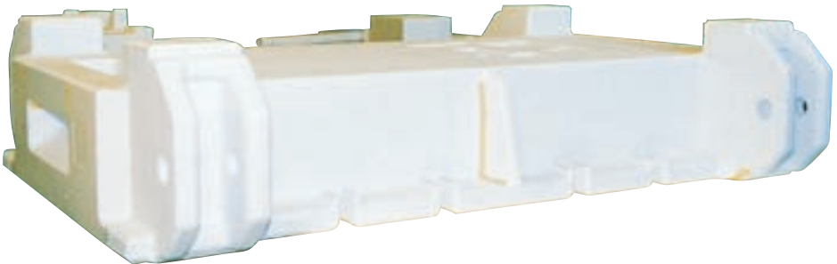
A model of foamed plastic, which is close to the shape of the component to save time in rough machining
