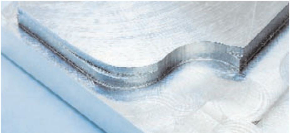
The upper pass on the component is machined with a machine control without sufficient look ahead function and it clearly shows that the corners have been cut, compared with the lower pass machined with sufficient look ahead function
