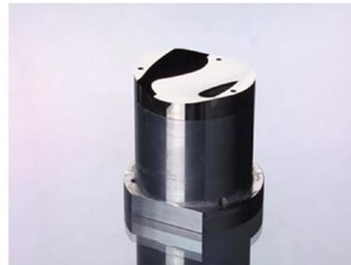
Mold insert for injection molding
