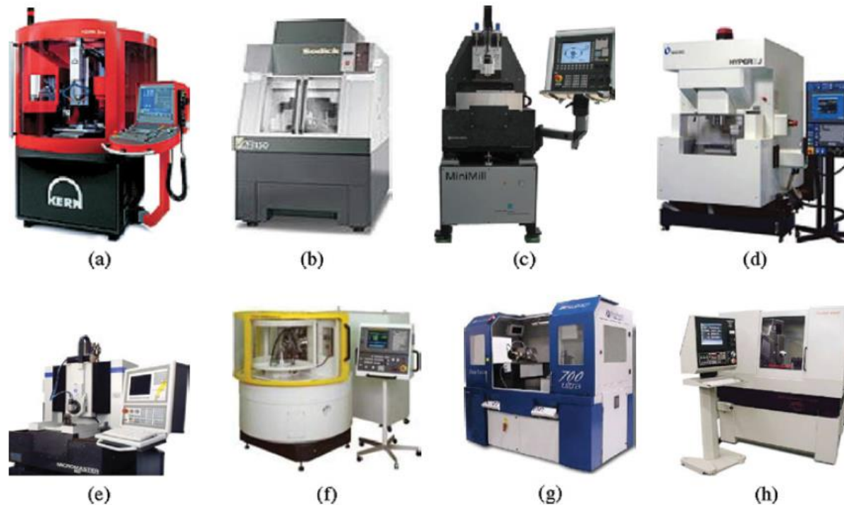
Figure 2.3 Industrial precision machine tools with micro cutting capability: (Reproduced from [2]) (a) Kern micro. Copyright KERN Microtechnik GmbH; (b) Sodick AZ150. Image courtesy of Sodick, Inc.; (c) Fraunhofer IPT Minimill. Reproduced from [6]; (d) Makino Hyper2J. Image courtesy of Makino; (e) Kuglar MicroMaster MM2. Image courtesy of Kugler GmbH; (f) Fanuc ROBOnano. Images courtesy of FANUC; (g) Precitech freeform 700 Ultra. Image courtesy of Ametek Precitech; (h) Moore Nanotech 350FG. Copyright Moore Nanotech
