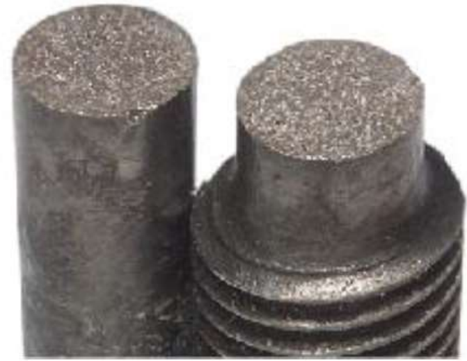
brittle fracture in a mild steel
