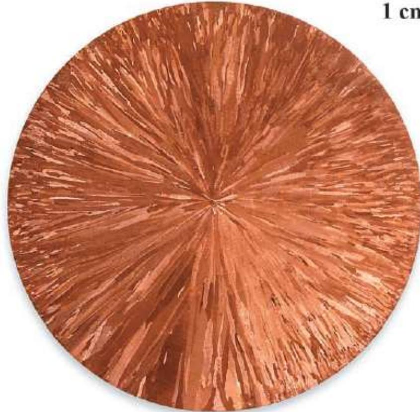
**Figure 4.12** Cross-section of a cylindrical copper ingot. The small needle-shaped grains may be observed, which extend from the center radially outward.
