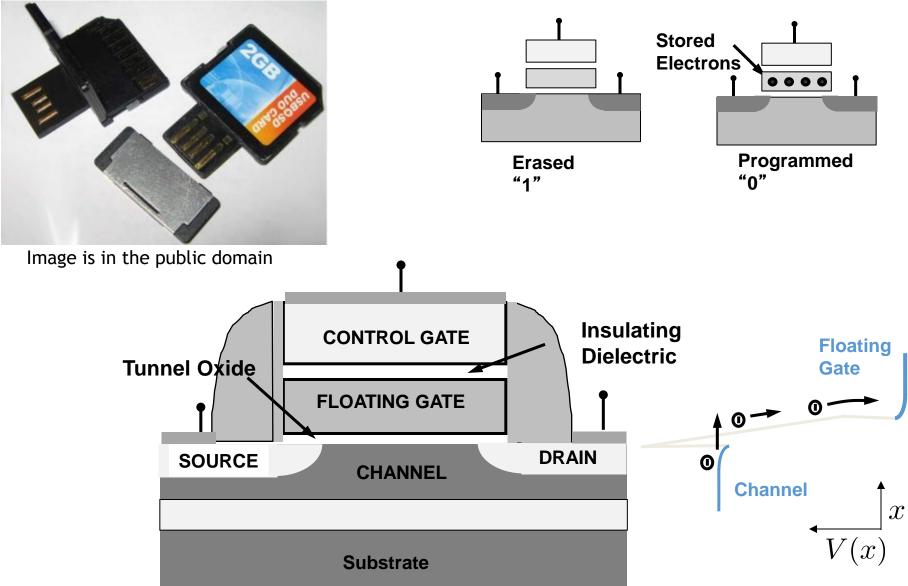
Electrons tunnel preferentially when a voltage is applied
