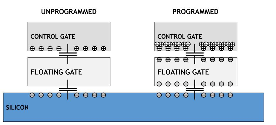
To obtain the same channel charge, the programmed gate needs a higher control-gate voltage than the unprogrammed gate
