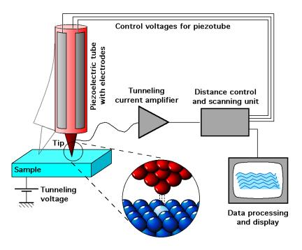
At this distance the coulomb force between the tip and an atom of the sample is actually enough to move the atom
