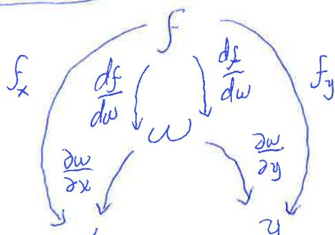
$$f_y = \left( \frac{df}{d\omega} \right) \left( \frac{\partial \omega}{\partial y} \right)$$
