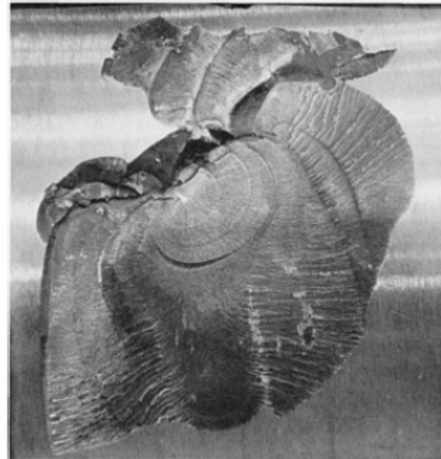
Fig. 57 Circular spall on the surface of a forged, hardened alloy steel mill roll. The arrow indicates the fracture origin. Note the fatigue marks showing the growth away from the origin, followed by brittle fracture. 0.68x
