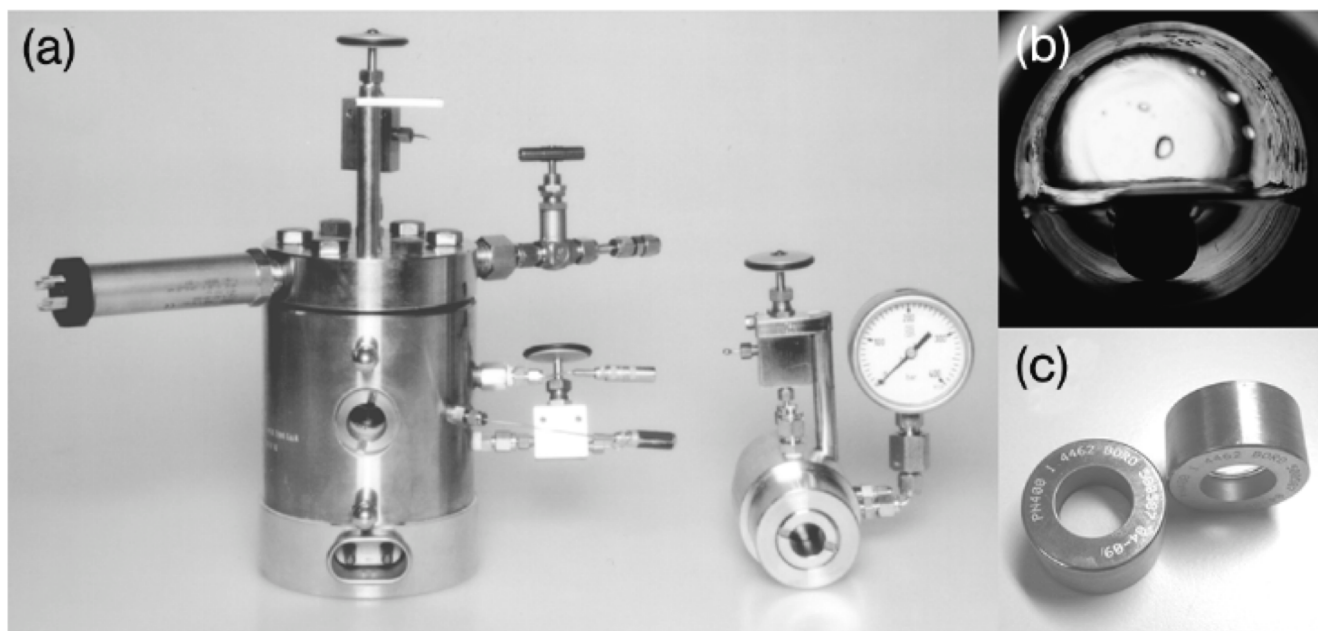
Figure 2.5 Window-equipped autoclaves (a), view through the windows of the autoclave (b), and metal fused high-pressure windows (c).
