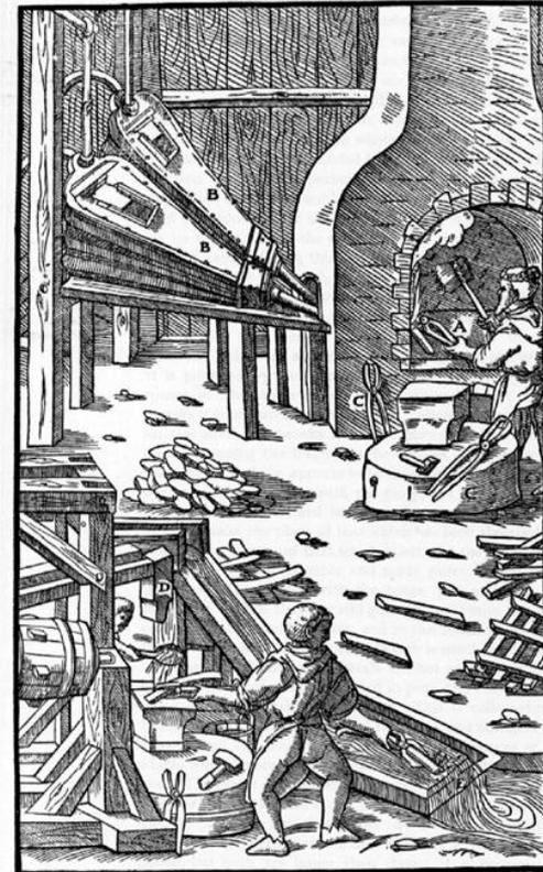
A—FORGE. B—BELLOWS. C—TONGS. D—HAMMER. E—COLD STREAM.
