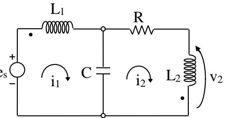
$$V_2(s) = -s|M|I_1 + sL_2I_2 \rightarrow v_2(t) = 7,54e^{-0,1563t} \cos(7,9041t - 174,35^\circ) H(t), \text{ (V, seg)}$$
