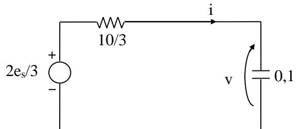
$$a) \quad G_1(s) = \frac{I(s)}{E_s(s)} = 0,2 \frac{s}{s+3} \quad \left( mS, \frac{1}{ms} \right)$$
