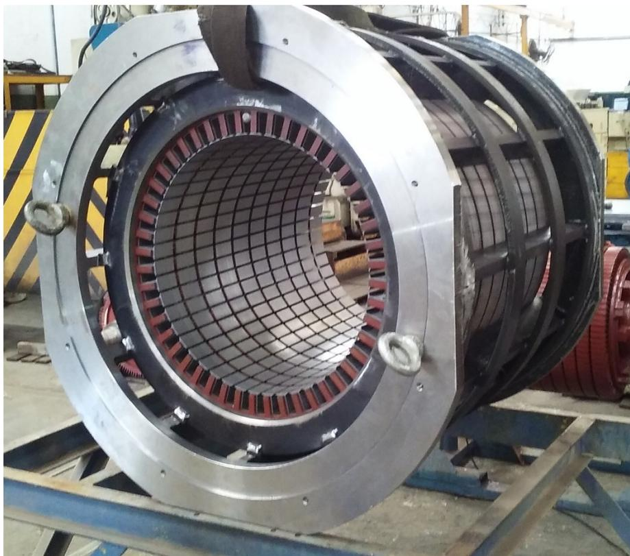
ESTATOR COM AS LÂMINAS DO
