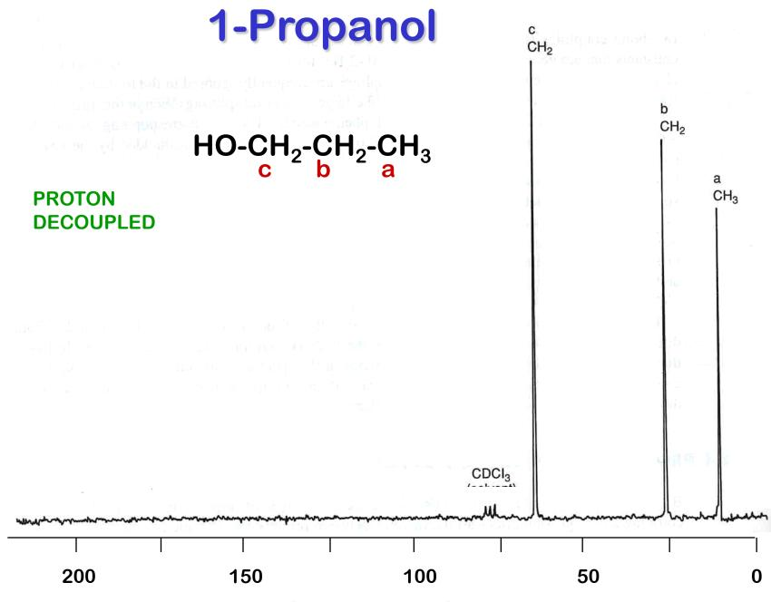
Proton-decoupled 13C spectrum of 1-propanol (22.5 MHz)
