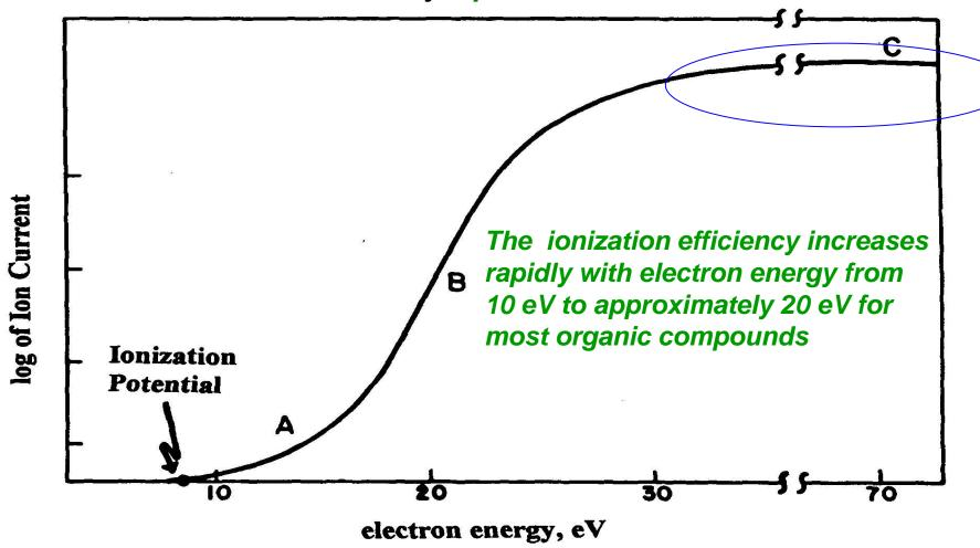
**FIG. 7.3.** Relationship between ion production and energy (electron volts) of ionizing electrons: region A, threshold region, principally molecular ions produced; region B, production of fragment ions becomes important; region C, routine operation, mostly fragment ions.
