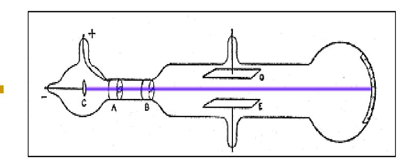
Schematic drawing of Thomson's apparatus in the experiment. Rays from the cathode (C) pass through a slit in the anode (A) and through a slit in a grounded metal plug (B). An electrical voltage is established between aluminum plates (D and E), and a scale pasted on the outside of the end of the tube measures the deflection of the rays.
