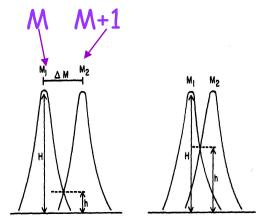
FIG. 1.4. Graphic representation of unit resolution with 15% valley (h/H) definition (left) and 50% valley definition (right).
