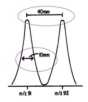
FIG. 1.5. Graphic representation of resolution using peak-width definition: full width at half maximum (FWHM). In this case, the separation of the peak centers is equivalent to four peak widths at half maximum (height).
