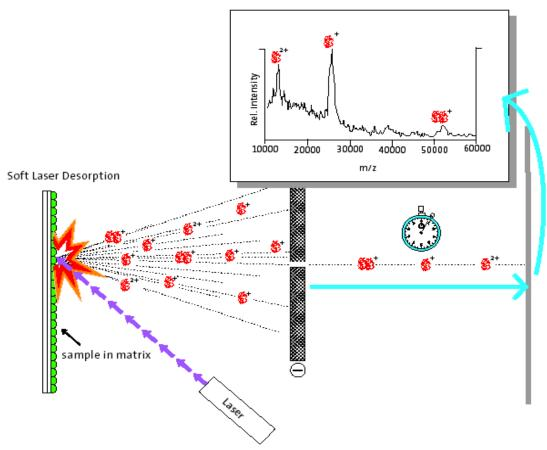
Figure 2. The soft laser desorption process.
