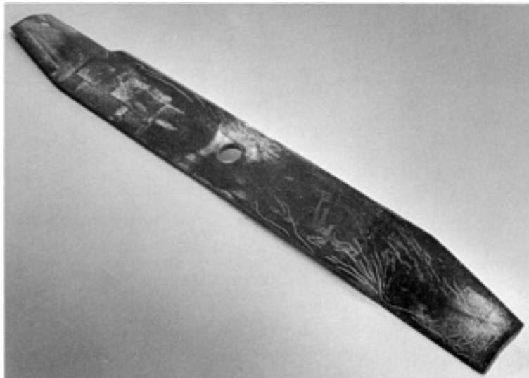
Fig. 24 Potentially dangerous cracks in a lawn mower blade revealed when fluorescent magnetic particles are exposed to black light. Courtesy of Magnaflux Corporation
