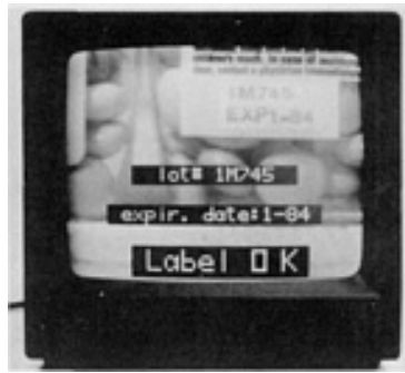
Fig. 15 Monitor screen of a machine vision inspection system verifying the expiration date and lot code on a pharmaceutical bottle. Courtesy of Cognex Corporation
