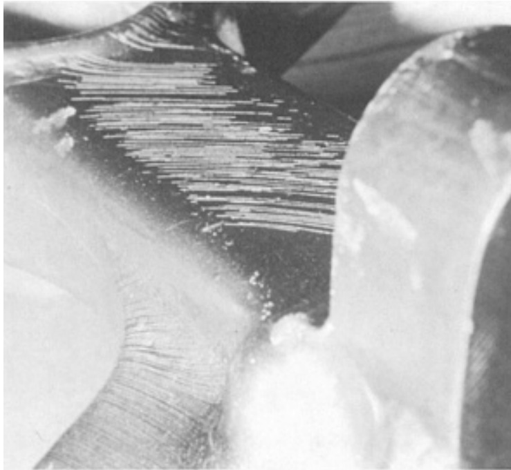
Fig. 8 Cracks in a brittle coating normal to the maximum tensile strains
