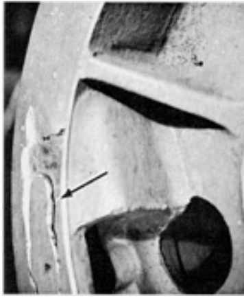
Fig. 31 Cold shut (at arrow) in the flange of a machined cast drum. Magnetic particle inspection revealed faint indications of the cold shut in the rough casting.
