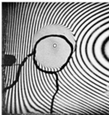
Fig. 4 Optical holographic interferogram of a pressure-stressed honeycomb-core sandwich panel. The sandwich panel was stressed by the atmospheric pressure of the air sealed in the core cavities when the air surrounding the panel was evacuated. An area of debond between the core and the near faceplate (of aluminum) is indicated by the fringe pattern in the vicinity of the ink marks on the faceplate. The background fringes were caused by general movement of the faceplate during evacuation.
