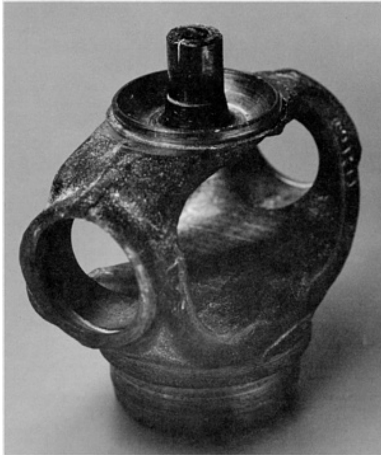
Fig. 26 Black light used to reveal magnetic particle indication of a crack in the centering stud of a ball-yoke-type universal-joint section of a drive-shaft assembly. Courtesy of Magnaflux Corporation
