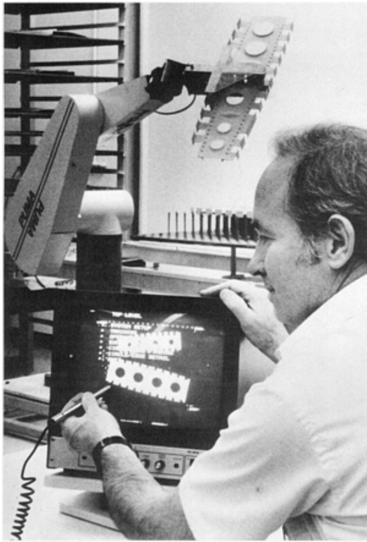
Fig. 20 Robot gripper arm used to maneuver and orient an aluminum aircraft section with the aid of a video camera that helps it see the workpiece and then identifies it from a data base. Courtesy of Lockheed-California Company
