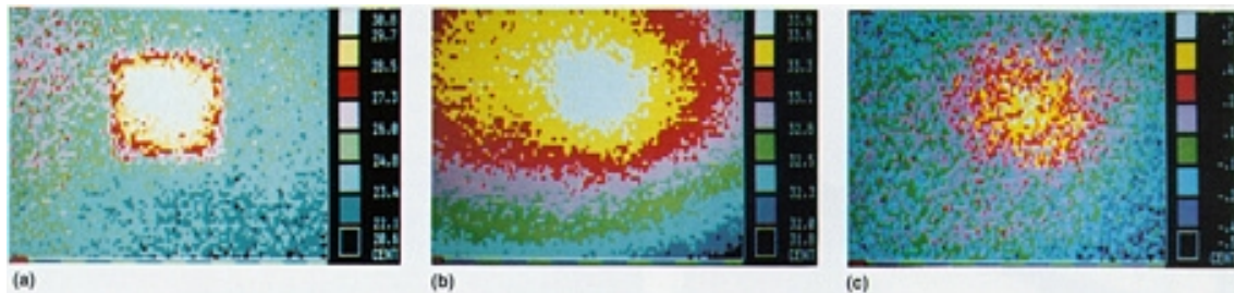
Fig. 17 Thermal images of graphite-epoxy sheets with 20 × 20 mm implanted Teflon defects at 0.3 mm depth (a) and 2.25 mm depth (b). Image processing (c) improved the detectability of the 2.25 mm depth defect. (P. Cielo, National Research Council of Canada)
