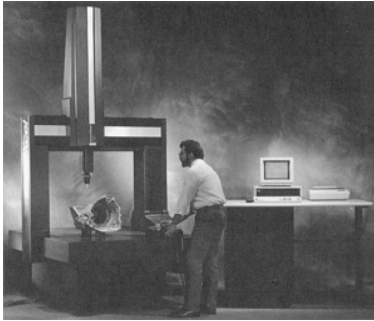
Fig. 5 Vertical moving-bridge CMM, which incorporates a granite base, inspecting a cast aluminum alloy four-wheel-drive transaxle gear case. The DCC motor drive that controls all of the axial movements is equipped with a remote joystick controller.
