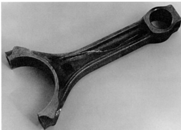
Fig. 27 Black light used to reveal magnetic particle indication of a lap that could lead to potential failure of a forged connecting rod. Courtesy of Magnaflux Corporation
