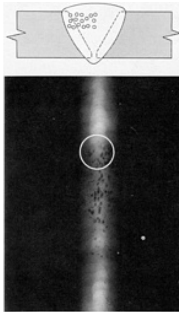
Fig. 27 Cluster porosity, which involves rounded or slightly elongated voids grouped together. Radiographic image: Rounded or slightly elongated darker-density spots in clusters with the clusters randomly spaced. Welding process: SMAW. Source: E.I. Du Pont de Nemours & Company, Inc.
