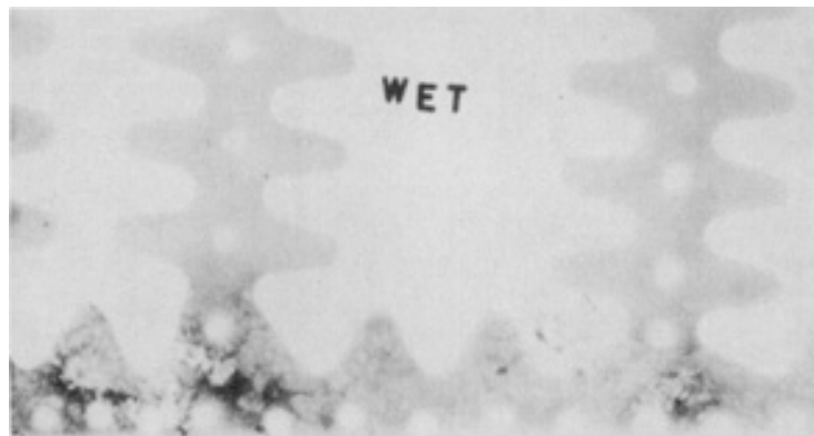
Fig. 19 Positive print from x-ray radiograph showing interface corrosion of an adhesive-bonded aluminum laminate
