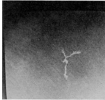
Fig. 10 Ti-6Al-4V \alpha - \beta processed billet illustrating the macroscopic appearance of a high-aluminum defect. 1.25 \times
