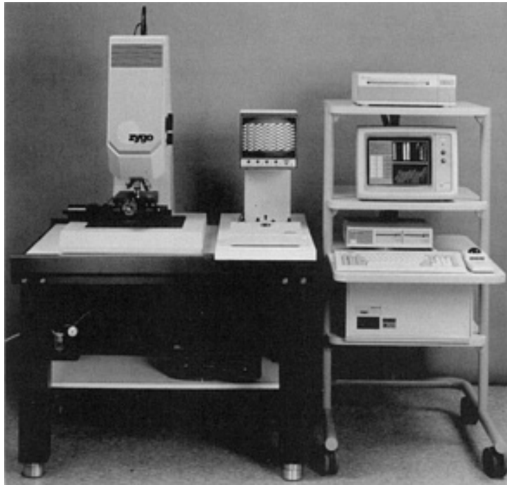
Fig. 11 Laser interference microscope with displays. Fizeau and Mirau interferometers are mounted in the turret.
