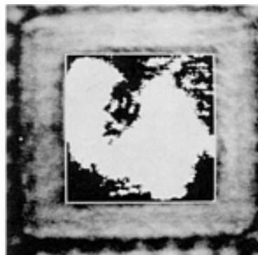
Fig. 30 Computer-analyzed SLAM acoustic image of Fig. 29 in which the disbonds are clearly displayed as
