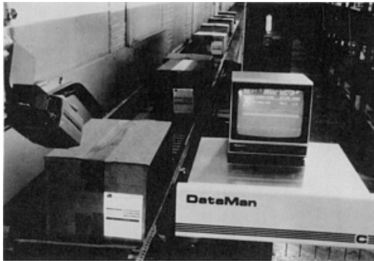
Fig. 16 Machine vision system reading box labels for sortation in a shipping facility. Courtesy of Cognex Corporation
