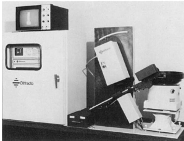
Fig. 21 Noncontact digital computer-vision-based fastener inspection system used to gage and then sort parts. Unit measures 11 parameters for up to 24 different fasteners that are stored in a memory and is capable of sorting up to 180 parts per minute or over 10,000 parts per hour. Courtesy of Diffracto Limited
