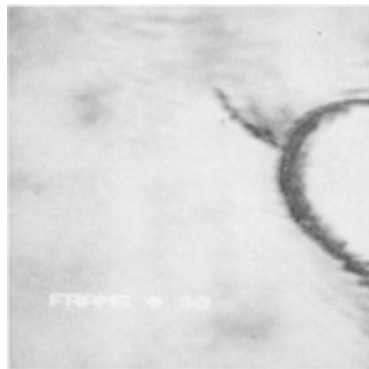
Fig. 16 100-MHz SLAM acoustic micrograph of an alumina panel section that contains a hole showing a crack with very high contrast. A digitally enhanced image of this alumina panel is also shown in Fig. 15 in the article "Use of Color for NDE" in this Volume. Field of view: 3 \times 2.25\text{ mm}
