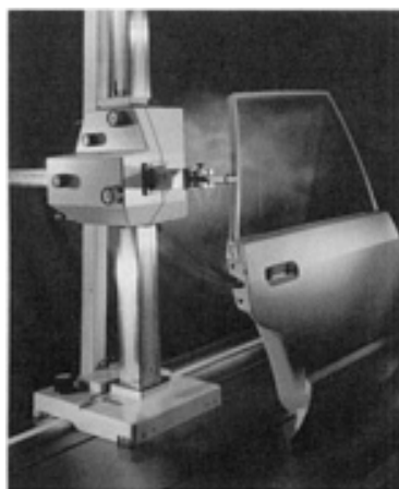
Fig. 10 Horizontal-arm fixed-table CMM using a metal scribing tool to inspect a steel sheet metal automotive door taken from the production line. This manually operated unit has a cast iron table.
