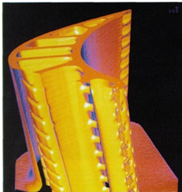
Fig. 7 Digital replica of a three-dimensional surface image of a turbine blade generated from computed tomography data (M.J. Dennis, General Electric NDE Systems and Services)
