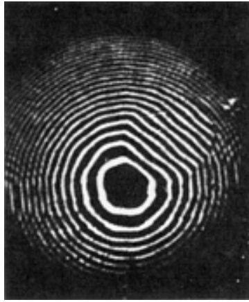
Fig. 15 Contour image of a spherical surface with one flat circular region (above center at right). Image was made at a frequency of 8 MHz using scanning acoustical holography. Each full fringe represents a change in elevation of 95\text{ }\mu\text{m} (0.00375 in.).
