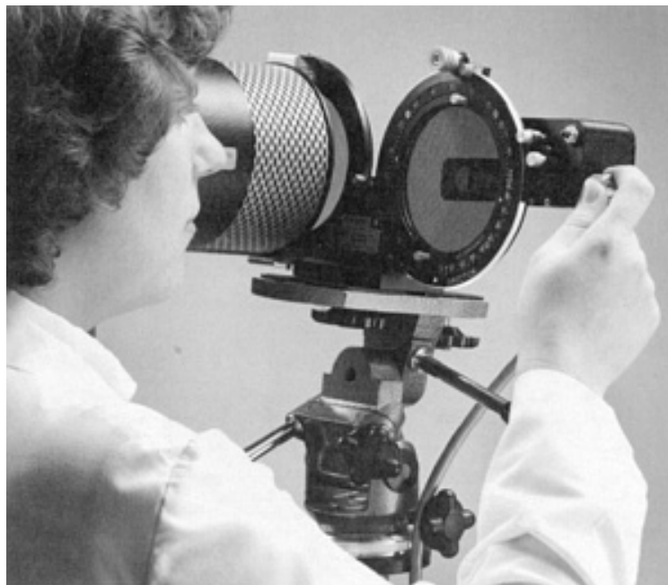
Fig. 5 Reflection polariscope with a null-balance compensator being adjusted by the operator
