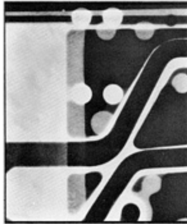
Fig. 63 Uneven wall thickness in an internal passage of a casting caused by core shift (top right). This radiograph, of an aluminum alloy casting about 3 to 6 mm ( \frac{1}{8} to \frac{1}{4} in.) thick, was made at 65 kV with an exposure time of 1 min.
