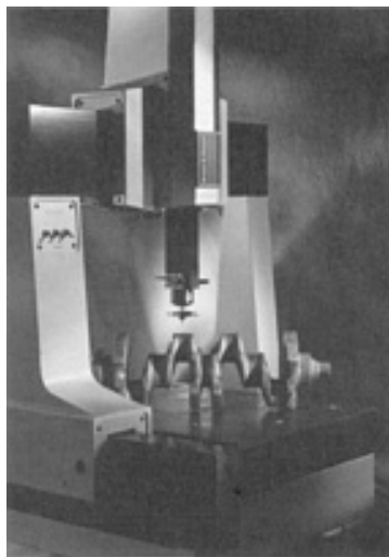
Fig. 4 Vertical moving-bridge CMM inspecting a case-hardened cast steel automotive crank-shaft using a touch-trigger probe. This manually operated unit has a granite table.
