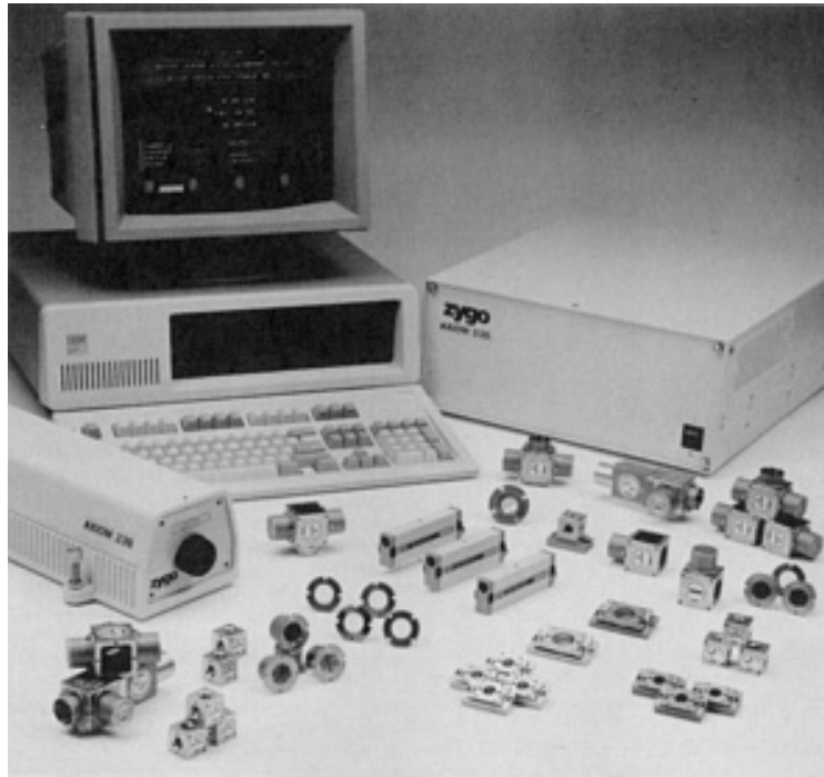
Fig. 6 Components of a laser interferometer. The components include a laser head, beam directing and measuring optics, receivers, electronic couplers, and a computer system.
