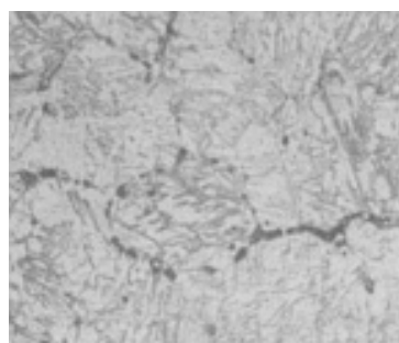
Fig. 3 Replica showing random and linked microvoids in the heat-affected zone of a secondary superheater outlet header weld. 400 \times . Courtesy of H.I. Newton, Babcock & Wilcox
