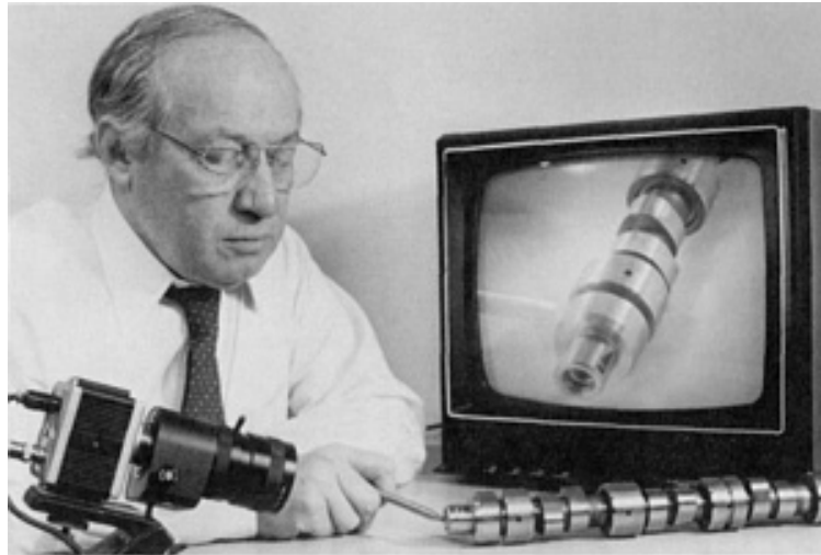
Fig. 18 Machine vision system that controls a multiple-programmed cam grinder being used to identify each specific automotive camshaft to determine machine settings. Courtesy of Industrial Automation Systems, Gould, Inc.
