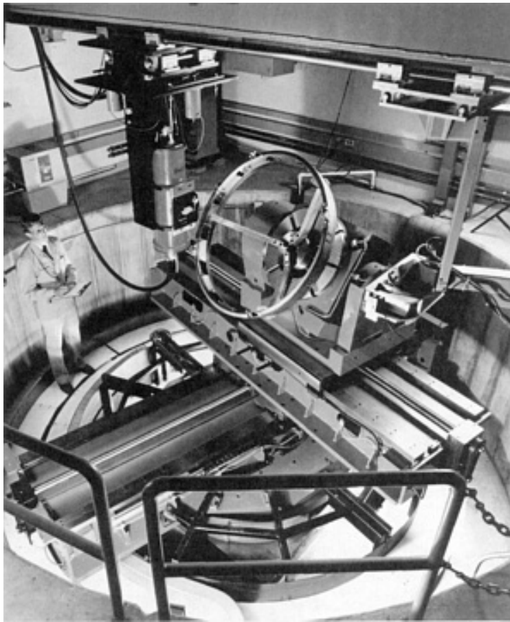
Fig. 16 Industrial computed tomography system x-ray cell for the inspection of large fabricated components and castings with multiaxis parts manipulator
