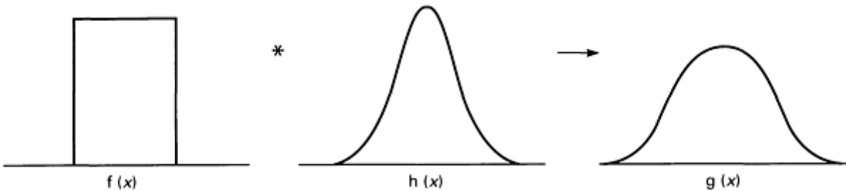
Fig. 29 Convolution operation (*) in which a distribution f(x) is blurred by a function h(x) to form the blurred distribution g(x) . The function h(x) is analogous to the PSF of an image system or a smoothing convolution filter in image processing.
