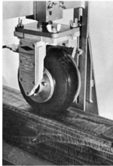
Fig. 53 Mechanized setup for the pulse-echo ultrasonic inspection of steel billets using a 250 mm (10 in.) diam wheel-type search unit and a longitudinal wave straight beam at 0° angle of incidence
