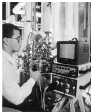
Fig. 11 Operator viewing a weld 21 m (70 ft) inside piping with a videoscope. Courtesy of Olympus Corporation
