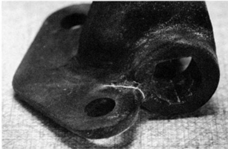
Fig. 23 Casting viewed under black light showing strong magnetic particle indication with minimal background fluorescence. Courtesy of Magnaflux Corporation
