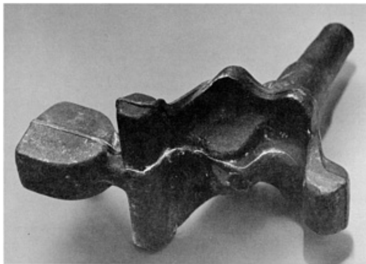
Fig. 19 Spindle defects revealed with water-base magnetic particle testing. Courtesy of Circle Chemical Company
