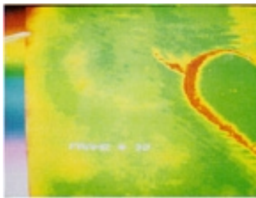
Fig. 15 100-MHz SLAM micrograph of the alumina panel shown in Fig. 16 in the article "Acoustic Microscopy." Color is used to delineate a crack with a specific acoustic brightness level. (L.W. Kessler, Sonoscan, Inc.)
