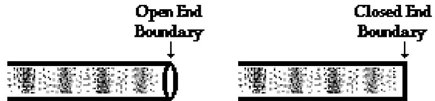
The open end of a cylindrical tube serves as a "free end reflector" and the closed end of a cylindrical tube serves as a "fixed end reflector."
