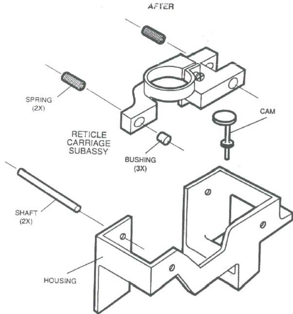
**Figure 1.12** Reticle assembly—new design. (Courtesy Texas Instruments, Inc.)
