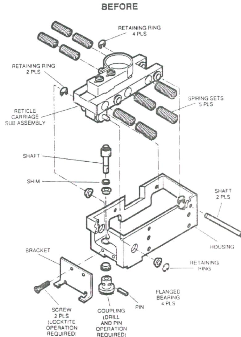
Figure 1.11 Reticle assembly—original design. (Courtesy Texas Instruments, Inc.)
