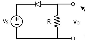
Respostas: c)  $\theta = 172^\circ$  ; d)  $v_{O\acute{m}e\acute{d}io} = -2,84V$  ; e)  $i_{Dpico} = 4,65mA$  ; f)  $V_{Rev} = -10V$
