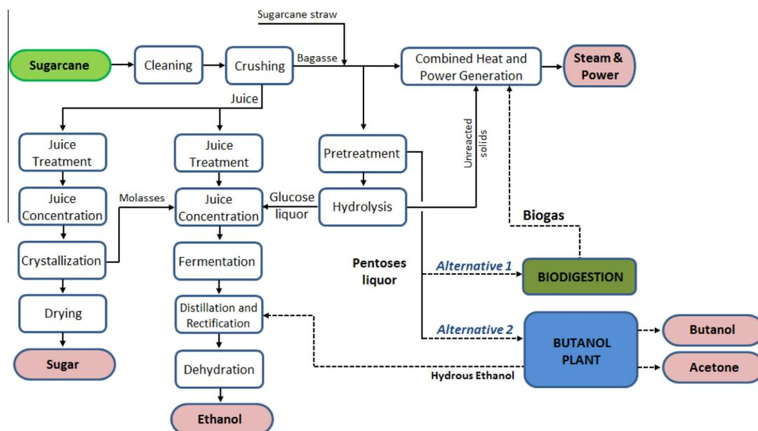
**Fig. 1.** Schematic diagram of an integrated 1G–2G sugarcane biorefinery with sugar, power, and ethanol production (ethanol from sugarcane juice and hexoses from bagasse). Alternatives for pentoses use: (1) biodigestion of pentoses – resulting biogas is used for power and steam generation; (2) fermentation of pentoses for production of butanol, and the by-products acetone and hydrous ethanol.
