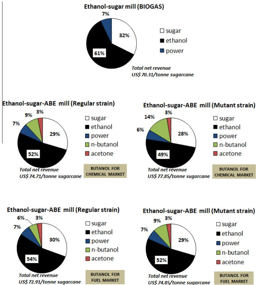
Fig. 4. Revenue breakdown for each biorefinery scenario.
