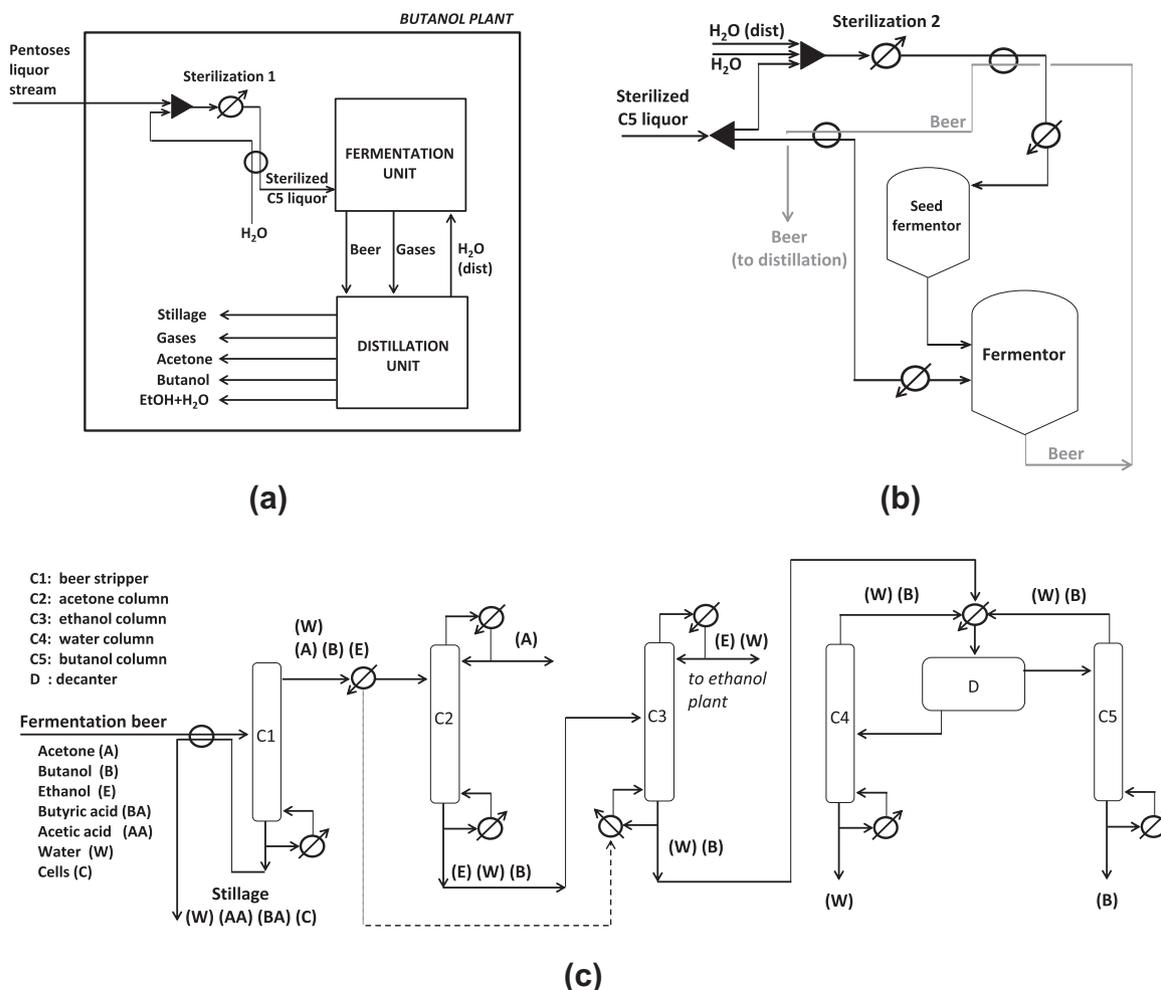
**Fig. 2.** Butanol plant (fed with pentose sugars from sugarcane biomass) simulated in Aspen Plus®. (a) Hierarchy blocks corresponding to fermentation and distillation units inserted in the Virtual Sugarcane Biorefinery (VSB, developed by CTBE). (b) Fermentation unit. (c) Distillation unit.
