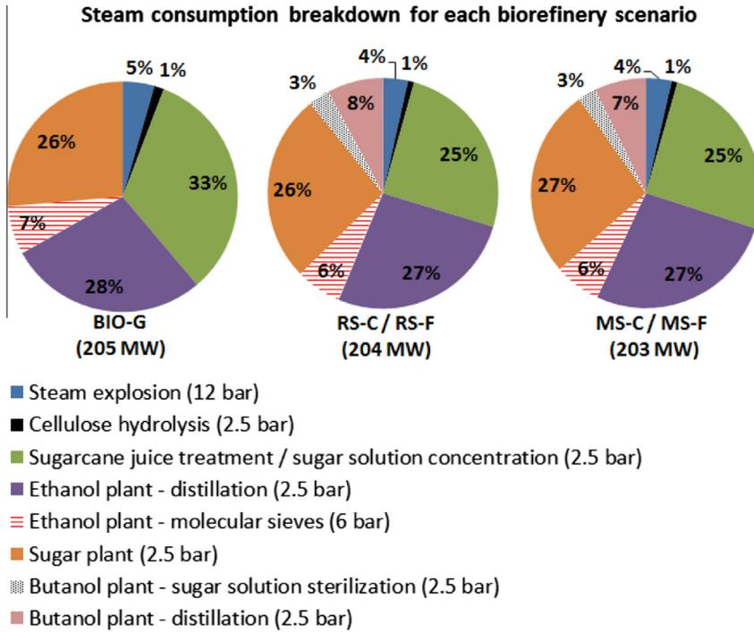
Fig. 3. Steam consumption breakdown for each biorefinery scenario.
