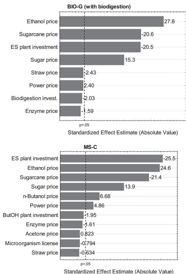
Fig. 5. Sensitivity analysis. Pareto charts of the effects of economic parameters on IRR for biorefinery scenarios BIO-G and MS-C. ES plant stands for the investment in the biorefinery considering neither biodigestion unit nor butanol plant (ButOH plant).
