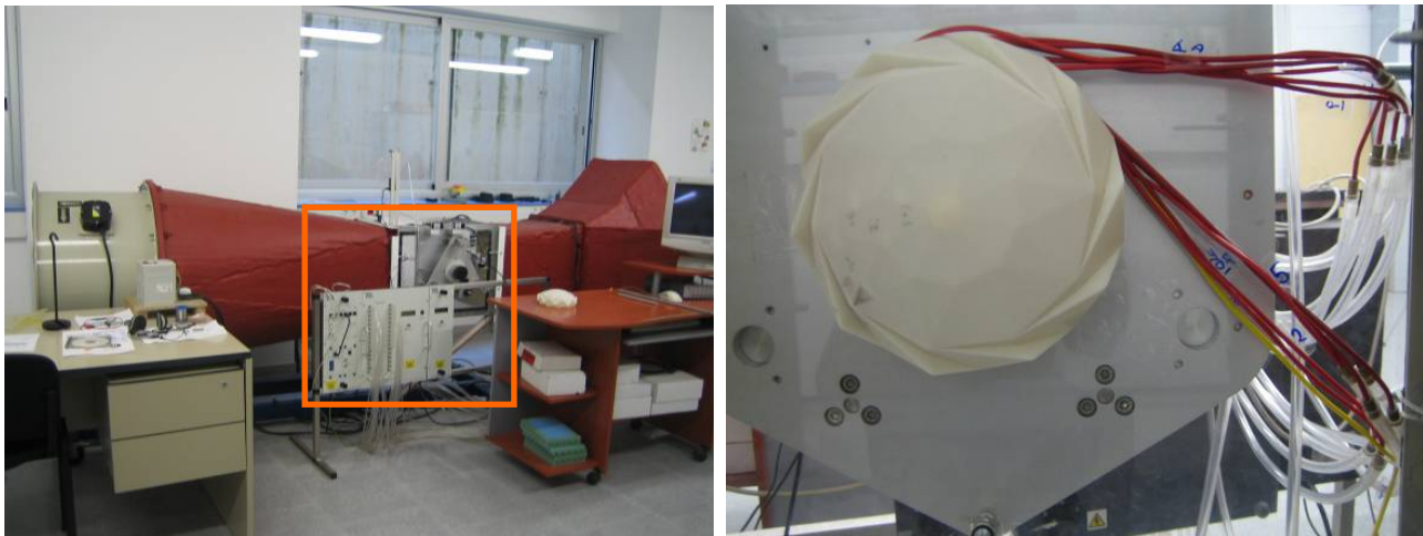
Figure 11. Wind-tunnel testing – scale model 1:250
