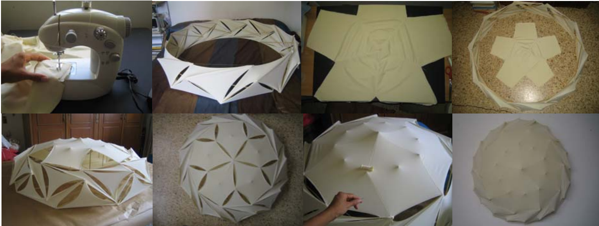
Figure 9. Tensegrity dome with a diameter of 100 cm – scale model 1:100
