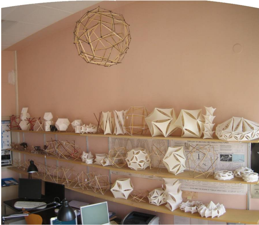
Figure 2. Examples of sixty scale models in tensegrity. Models developed using an intuitive and experimental method based on the geometry.
