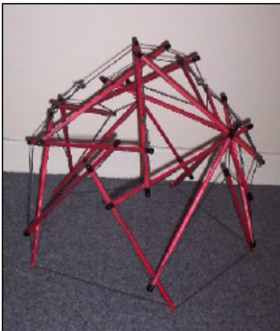
Fig. G.15. "Dome from Truncated Icosahedron" (1/2) Model made by the author (2004)
