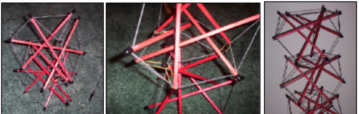
Fig. G.4. Assembly of Truncated Tetrahedron by strut-cable contact.
