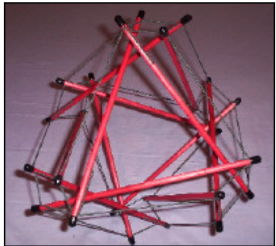
Fig. G.2. “Tensegrity Truncated Octahedron”
