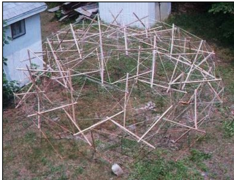
Fig. 6.6. "8v Double-Layer Tensegrity Dome" Model built and published by Burkhardt (1999-2004)
