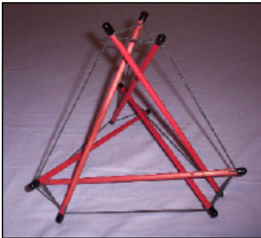
Fig. G.1. “Tensegrity Truncated Tetrahedron”
