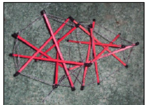
Fig. G.3. Assembly of two Truncated Tetrahedron by strut-strut contact.
