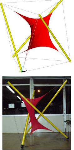
Figure 3. Comparison between the final *Ansys* finite element model, incorporating the tensegrity module, the membrane and the connecting cables, with the real sculpture.
