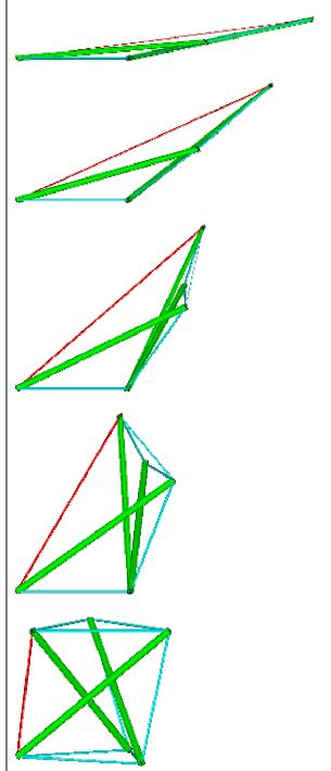
Figure 2. Numerical simulation of the assembling of the tensegrity module.
