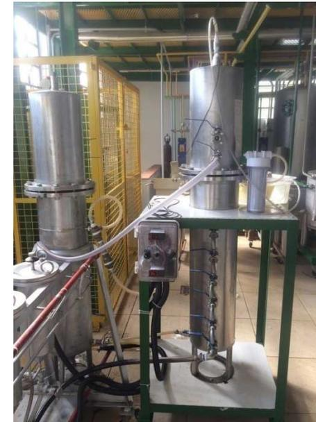
Figura 8: Reator UASB
