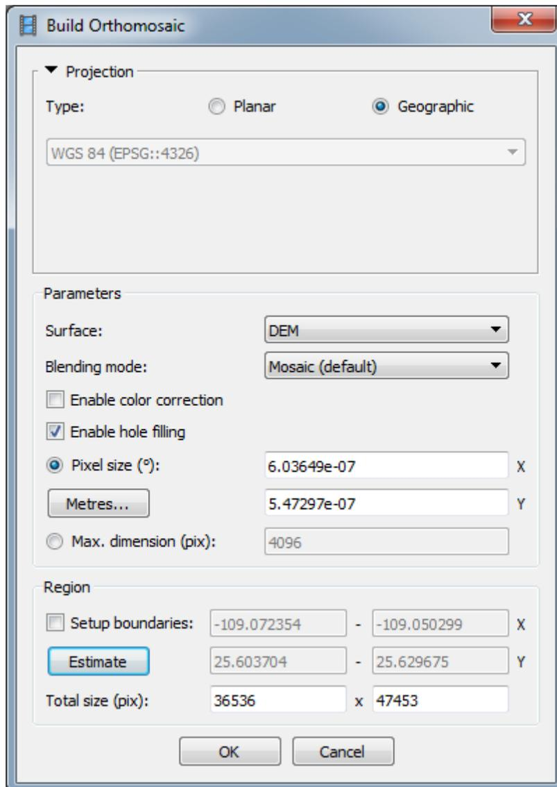
Select desired surface for orthomosaic generation process: mesh or DEM, and blending mode.
