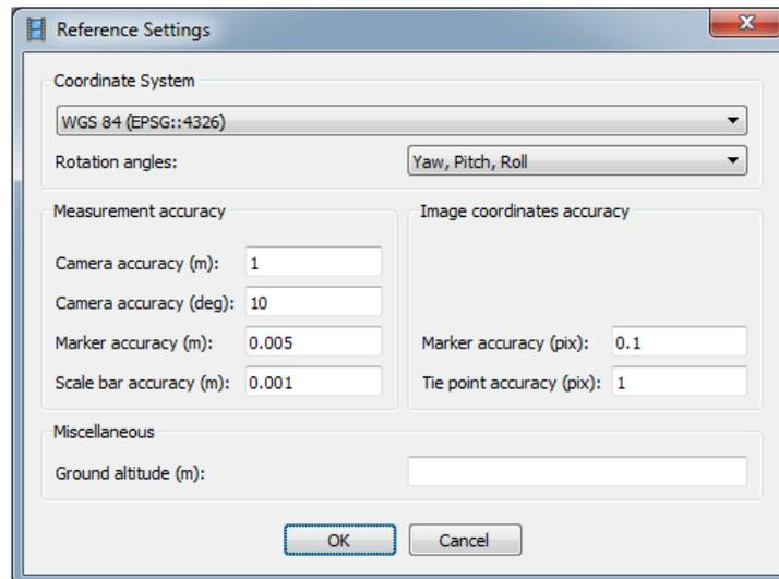
**Camera accuracy (m):** 1 (specify value according to the measurement accuracy).
