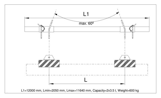
The lifting beam has been designed to transfer the hollow core slabs in construction sites.
