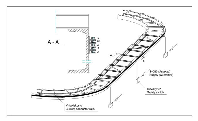
The current conductor rails supply energy to the concrete distribution shuttle. The rail system is dimensioned according to the power requirement and the length of the track. The rails are fastened to the track constructions.
