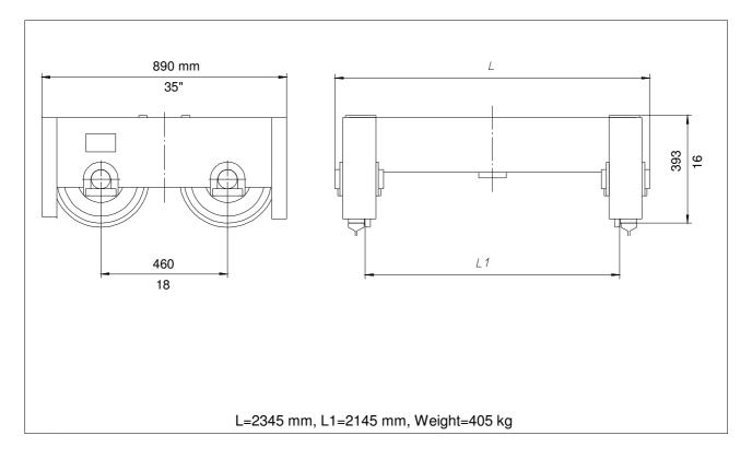
The transport wagons are used for transporting of precast units from the hall to the storage area.
