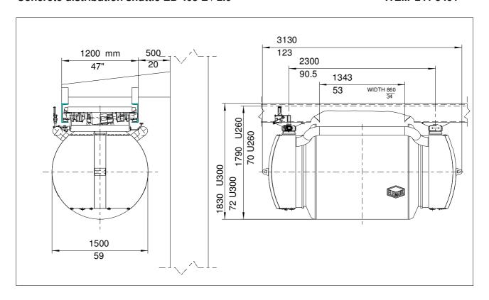
The concrete distribution shuttle has been designed for concrete distribution on a two-rail track from the batching and mixing plant to an intermediate silo or to a casting machine. The concrete distribution shuttle is suitable for straight and curved tracks.
