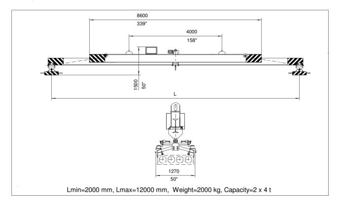
The lifting beam has been designed to transfer the hollow core slabs from the pallets inside the plant.
