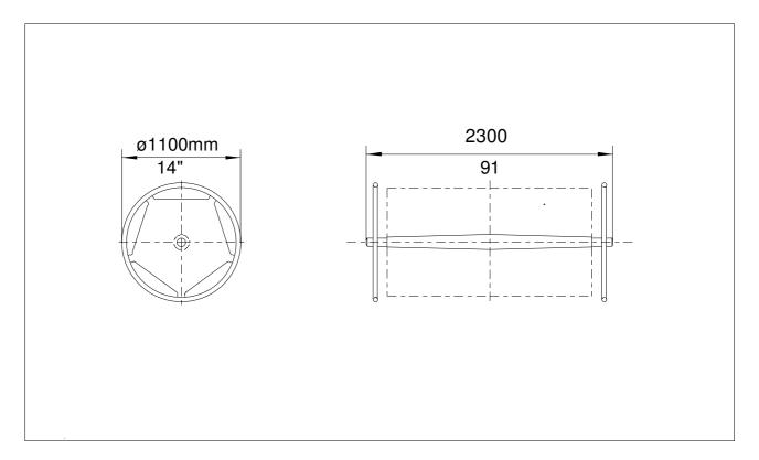
The cover roll makes the handling of the HC-slab cover easier.
