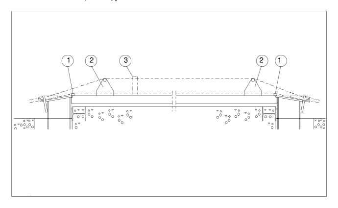
The strand comb serves for correct positioning of the stressing stands. The strand combs are located at both ends of the casting bed. The distance from the end of the casting bed depends on the height level of the upper strands (check angle of the strands). The comb for lower strands is located straight at the end of the bed.
