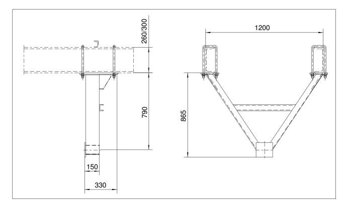
The end stopper for concrete distribution track EB 415 consists of a welded steel construction.
