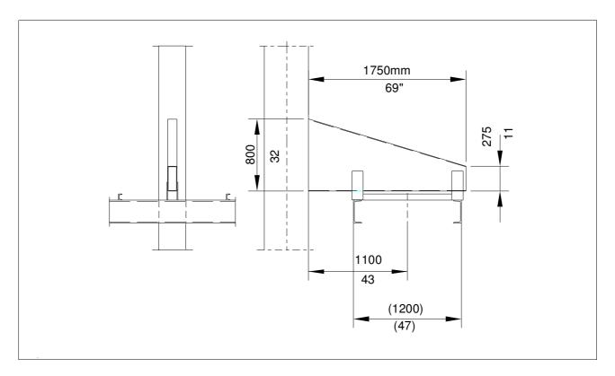
For supporting the concrete transport track, the consoles are fastened on columns by welding
