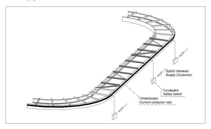
One feed point is needed for each track part. The division of the track into parts can be made from the maintenance point of view and/or according to the location. Target of the division is to form units that are clear to control, maintain and operate.
