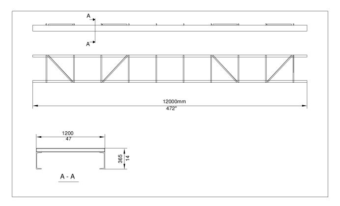
The track consists of a steel construction welded of two U-profiles and reinforced with cross and diagonal bracing.
