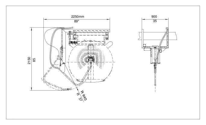
The washing station is designed for washing of concrete distribution shuttle.
