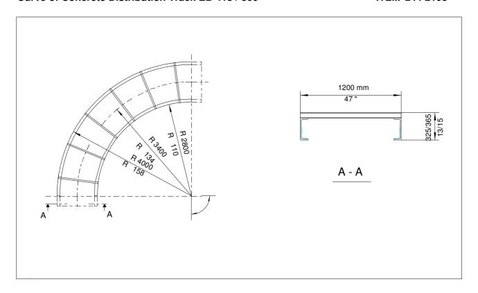
The track consists of a welded steel construction of two U-profiles reinforced with cross and diagonal bracing.
