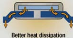
Figure 4. Cross-section of SO package with flip chip interconnect.
