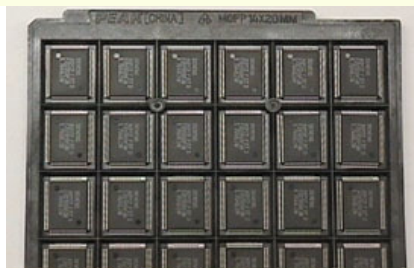
Figure 2. JEDEC tray with properly arranged units.
