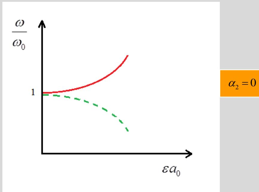
Frequency-amplitude curve ('backbone' curve)
