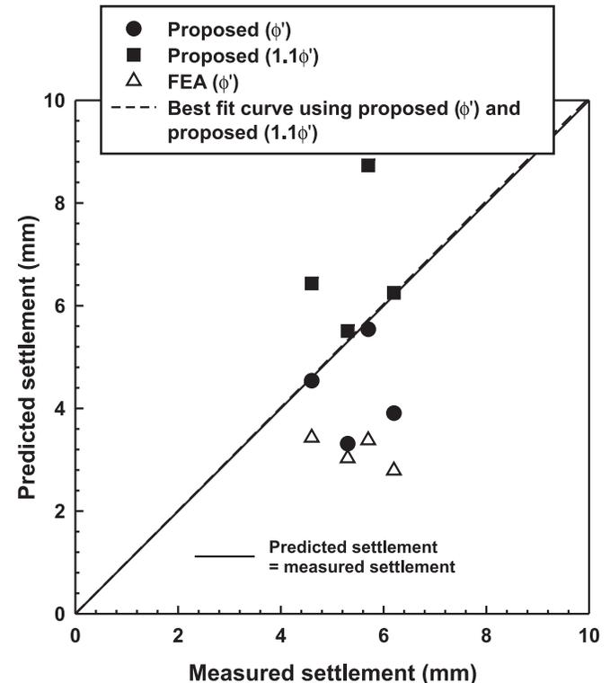
In addition to the proposed method, finite element analysis (i.e., FEA) was also carried out to show how the SVS relationship in unsaturated sands can be simulated using the elastic – perfectly plastic model.
