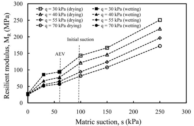
**Fig. 10.** Influence of wetting and drying history on resilient modulus (in series 3 tests).
