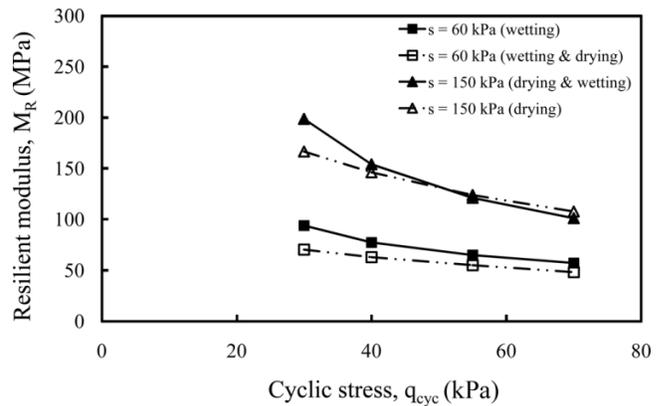
are probably because the bulk water effects dominate soil behaviour when suction is lower than the AEV of the soil (here about 60 kPa, see Fig. 3) in series 1 tests and meniscus water effects dominate soil behaviour when suction exceeds the AEV in series 2 tests (Ng and Yung 2008).
