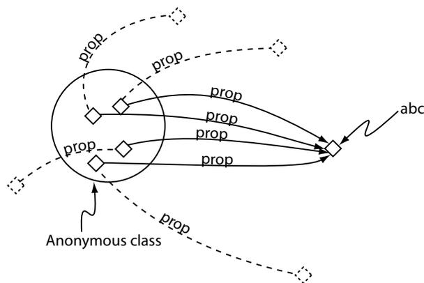
**Figure A.4:** A Schematic View Of The `hasValue` Restriction, `prop ∃ abc` — dashed lines indicate that this type of restriction does not constrain the property used in the `hasValue` restriction solely to the individual used in the `hasValue` restriction
