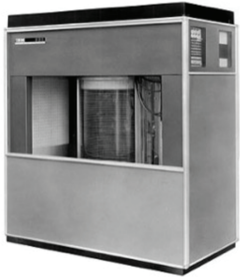
Figure 2-1: The spinning disk system for the IBM RAMAC 305
