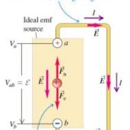
When a real (as opposed to ideal) emf source is connected to a circuit,  $V_{ab}$  and thus  $F_c$  fall, so that  $F_n > F_c$  and  $F_n$  does work on the charges.
