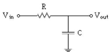
$$V_0 \sin[2\pi f t] = IR + \frac{Q}{C}$$
