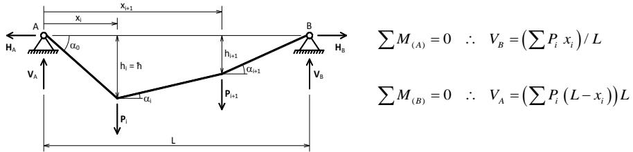
$$\left. \begin{array}{l} h_i = h^* \\ \sum M_{(i)}^{left} = 0 \\ \sum F_x = 0 \end{array} \right\} \Rightarrow H_A = H_B = \frac{V_A x_i}{h^*} = H \quad \text{'Thrust'}$$
