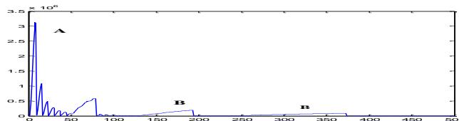
Transient of kinetic energy during the shape finding of a cable network via DR, with kinetic damping
