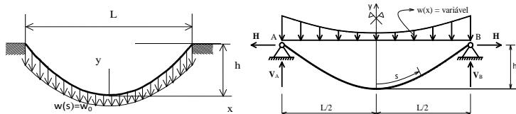
Inverting:  $s = \frac{H}{w_0} \sinh\left(\frac{w_0}{H} x\right)$  lenght of the catenary cable stretch  $[0, x]$
