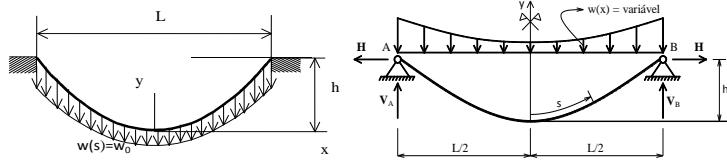
cable of homogeneous material and uniform cross-section ,  $w(s) = w_0$
