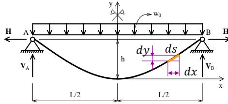
The length of a differential cable element is:  $ds = \sqrt{dx^2 + dy^2} = dx \left( 1 + \left( \frac{dy}{dx} \right)^2 \right)^{\frac{1}{2}}$
