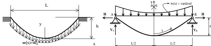
$$\text{But } ds = dx \left( 1 + \left( \frac{dy}{dx} \right)^2 \right)^{\frac{1}{2}} = dx \left( 1 + \left( \frac{w_0 s}{H} \right)^2 \right)^{\frac{1}{2}}$$
