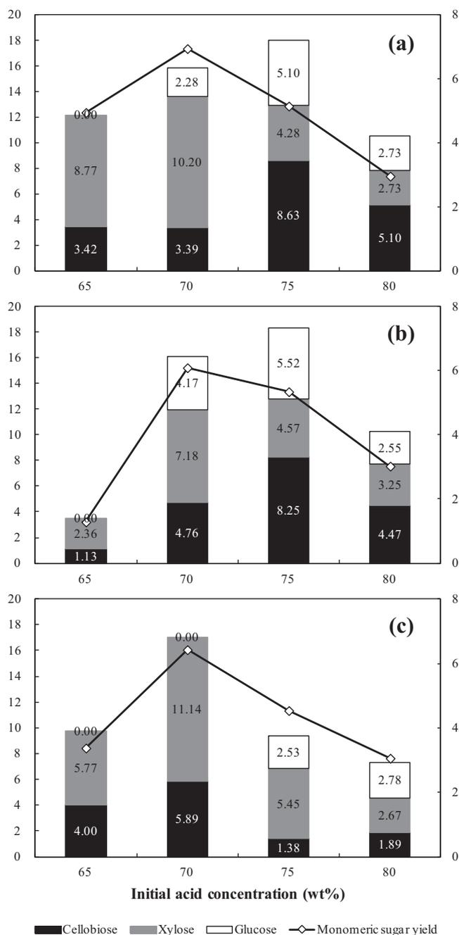
Fig. 3. Product distribution at the end of decrystallization reaction from: (a) oak wood, (b) pine wood, (c) EFB, at various initial acid concentration. The primary and secondary vertical axis represents sugar concentration (g/L) and monomeric sugar yield (wt%), respectively.
