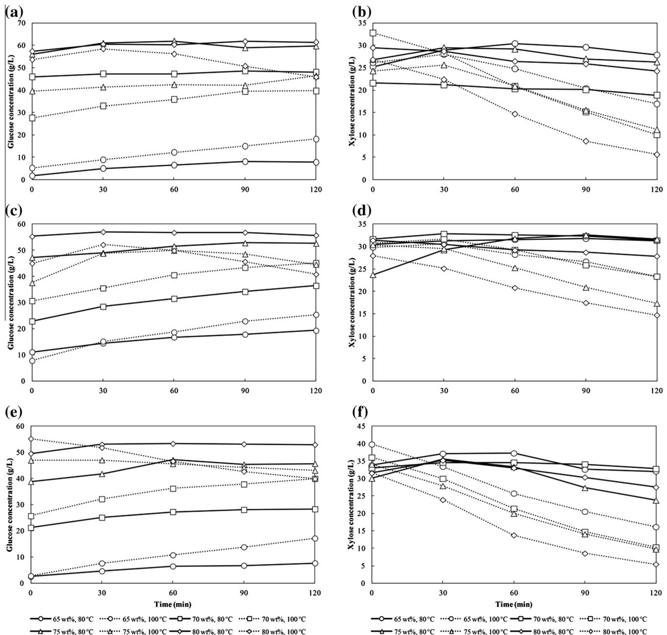
Fig. 5. Comparison of glucose and xylose concentration profile from the hydrolysis of: (a and b) oak wood, (c and d) pine wood, (e and f) EFB, at all process conditions.
