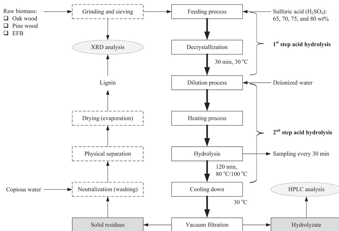
Fig. 1. Overall experimental process stages of the two-step concentrated acid hydrolysis.
