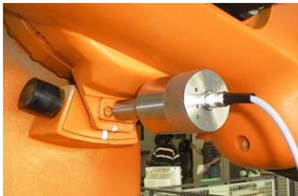
Fig. 5-5: EMT – electronic measuring tool
