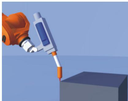
**Fig. 5-24: Origin of the base coordinate system**
