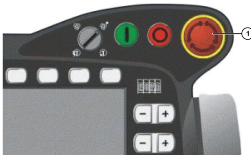
Fig. 3-3: EMERGENCY STOP button on the KCP
