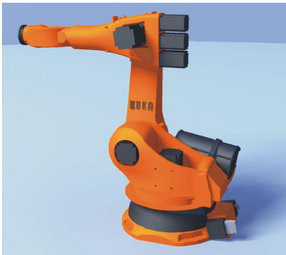
Fig. 5-2: Mastering position – approximate position
