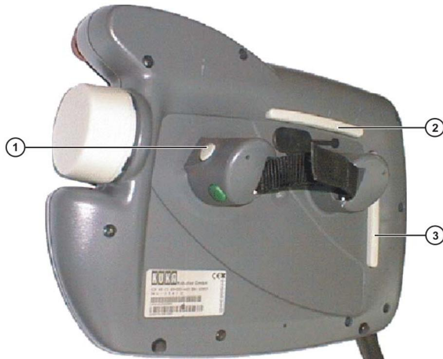
**Fig. 3-4: Enabling switches on the KCP**
