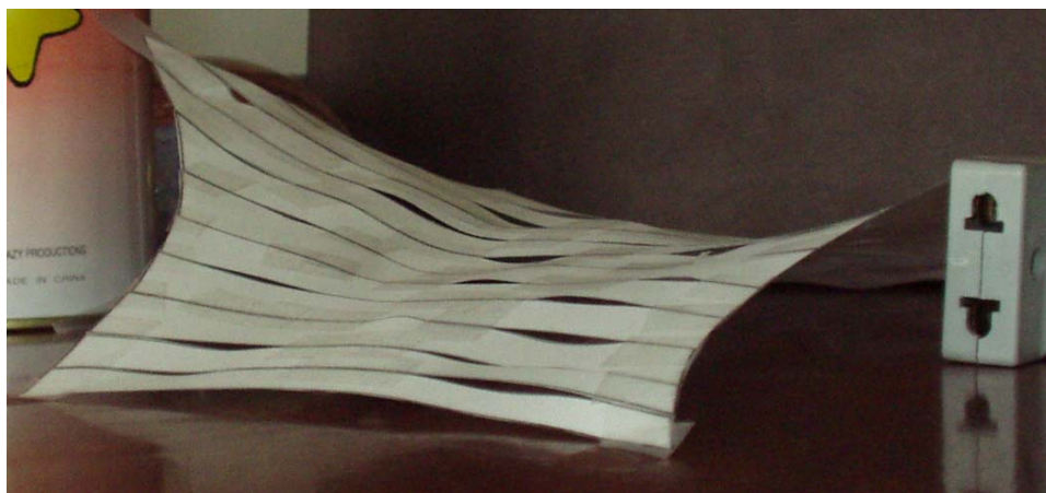
Figura 9. Assembling of a small scale, paper model, from flat patterns printed in an A4 sheet of paper.
