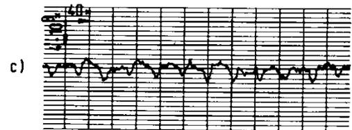
$R_a = 0.42 \mu\text{m}$  ,  $R_t = 3.21 \mu\text{m}$
