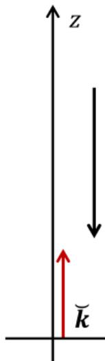
$$\left. \begin{array}{l} \frac{\partial p}{\partial x} = 0 \\ \frac{\partial p}{\partial y} = 0 \\ \frac{\partial p}{\partial z} = -\rho g \end{array} \right\} \implies p(z) = -\rho g z + cte$$
