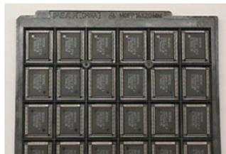
Figure 2. JEDEC tray with properly arranged units.
