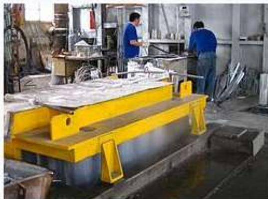
continuous hot vertical casting in process
