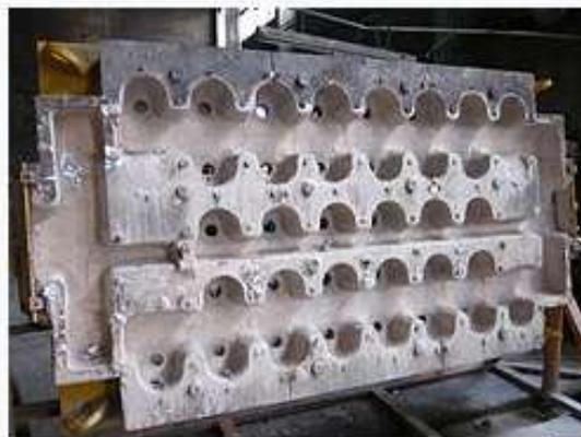
molten aluminum pours into this casting die
