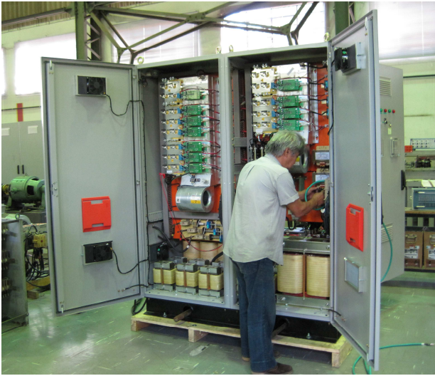
Figure 7: DVR test preparations at IEE-USP.
